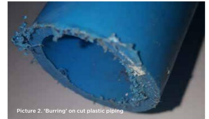
Picture 2. 'Burring' on cut plastic piping
