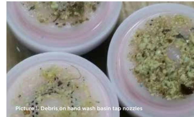
Picture 1. Debris on hand wash basin tap nozzles
