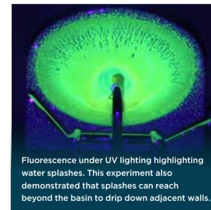
Fluorescence under UV lighting highlighting water splashes. This experiment also demonstrated that splashes can reach beyond the basin to drip down adjacent walls.
