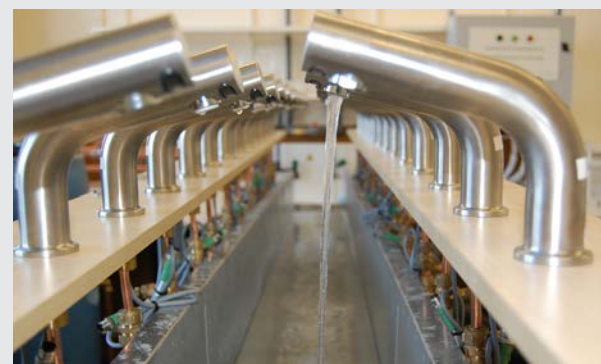
Porton Down experimental water distribution system (EWDS)
